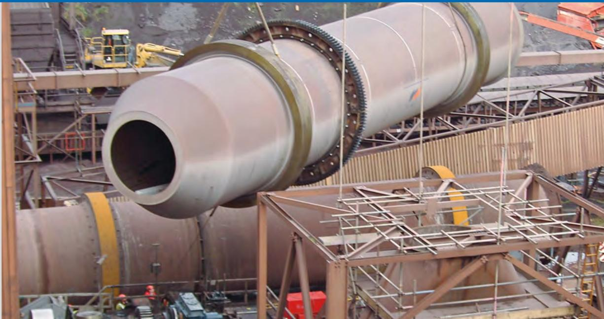
Sludge, especially that derived from mining operations, is granulated in a continuous process comprising two consecutive and continuous steps in which the sludge is mixed and granulated in the CEMTEC mixing/granulating drum.
