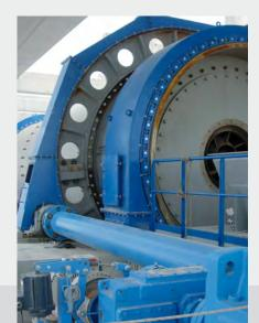
Depending on the fresh feed humidity, the cement mill can be equipped with a pre-drying chamber.
