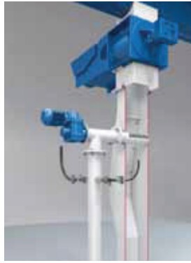
2 Typical installation of the Ceops sampling device at the process filter discharge chute
