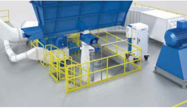
2 Typical installation of the Ceops sampling device at the process filter discharge chute
