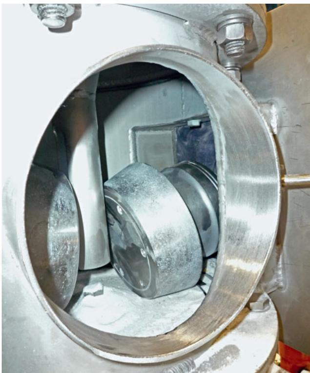
3 Blick in den Mahlraum • View into the grinding chamber
